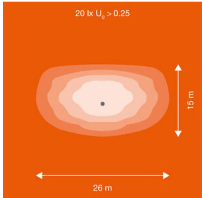
Streetlight Flex 80W RV25ST simplified isolux diagram
