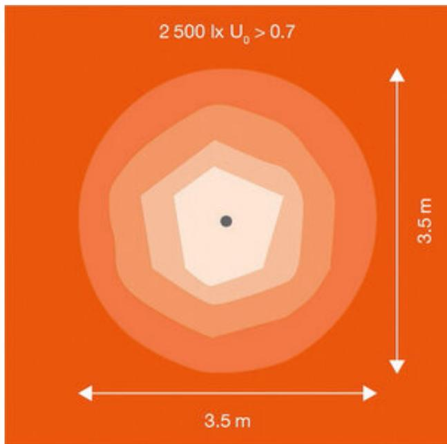
Floodlight Max 900W SYM 10 simplified isolux diagram
