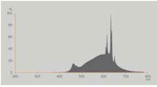
EPREL Data Spectral Diagram LEDr
