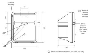
② 3 fixing positions screws, plugs and washers supplied
